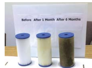
This is what a Sediment Pre-Filter does:
